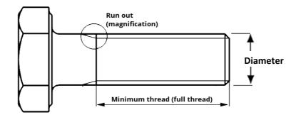
Thread Lengths On Longer Bolts Is Calculated By:
